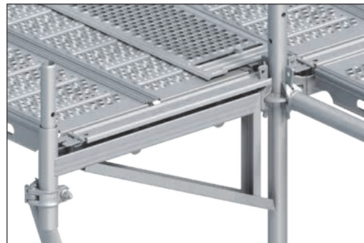
Assembly situation: U-console bracket LW , 0.73 m wide 1c (top) or alternatively U-ledger 0.73 m in conjunction with bracket brace 2.05 m 3 (left).
