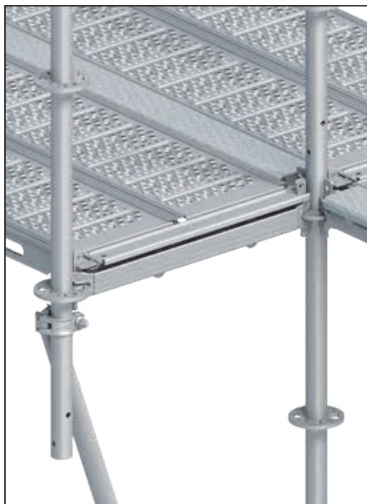
Assembly situation: U-console bracket LW , 0.73 m wide 1c (top) or alternatively U-ledger 0.73 m in conjunction with bracket brace 2.05 m 3 (left).
