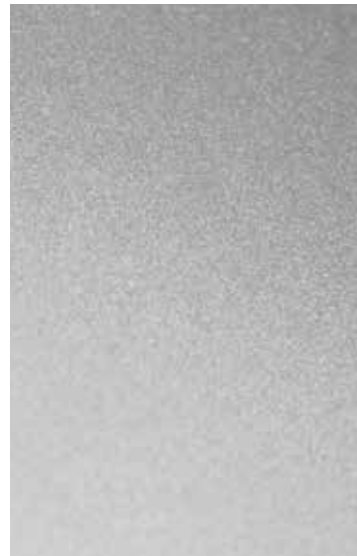
BEAD BLASTED – EVEN AND MATTE SURFACE
